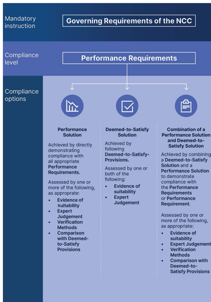
Figure C.1 Demonstrating compliance with the NCC
